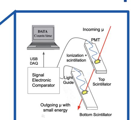
A portable compact muon detector is constructed at TDLI using plastic scintillators and photomultiplier tubes.
