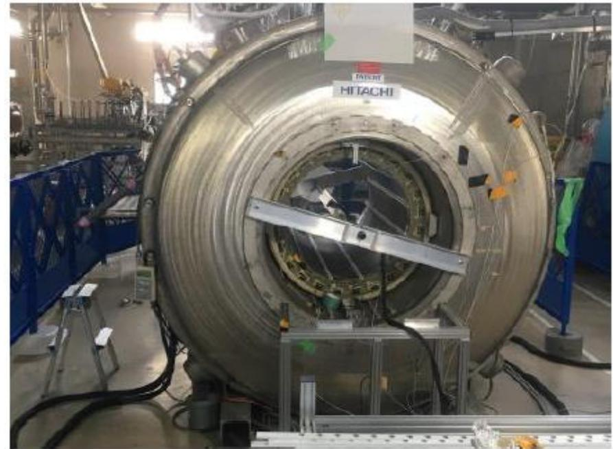
Superconducting magnet (1.7T)
