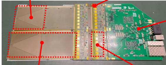
FPGA-based readout board (FRBS) for data/clock communication; prototype is being tested.
