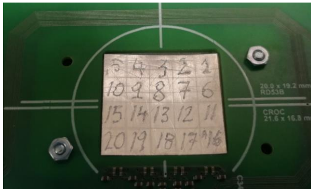
Aluminum foil placed in the backside of the module, divided into 20 smaller pieces
