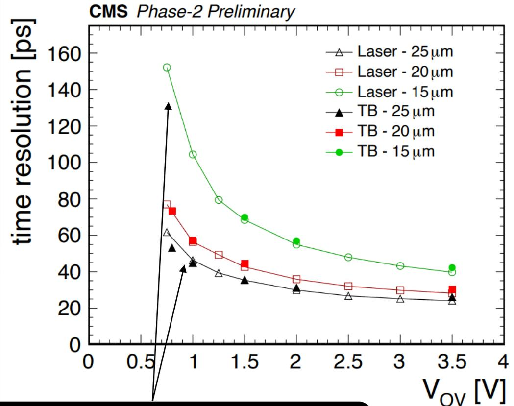
Electronic noise contribution reduced for large-cell SiPMs, as confirmed by lab tests
